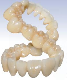
In order to put the specimen in even more severe environment than 1st step, twisting motion is added in 2nd step. Thermal expansion behavior changes from 2D to 3D. With 11 soldering and 17 firing in total, very high level technique was required just to make the model. There was no cracking occured to the end of the test.
