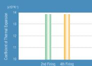
Fluctuation of Thermal Expansion by Repeated Firing
