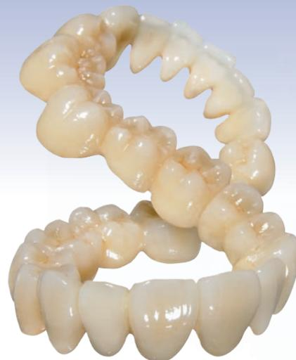
In order to put the specimen in even more severe environment than 1st step, twisting motion is added in 2nd step. Thermal expansion behavior changes from 2D to 3D. With 11 soldering and 17 firing in total, very high level technique was required just to make the model. There was no cracking occurred to the end of the test.
