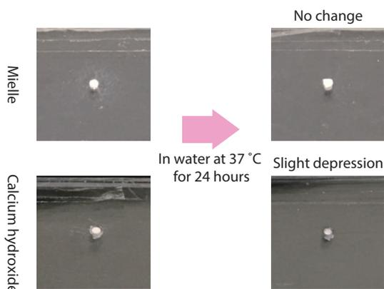
Figure 3-6 Changes in appearance before and after immersion in water
