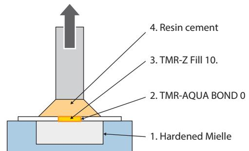
Figure 3-34 Structural Schematic Diagram of Adhesive Test Specimens
