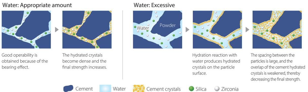
Figure 3-13 Schematic diagram of Mielle setting with appropriate and excessive water
