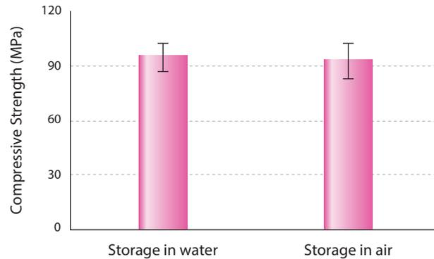
Figure 3-10 Compressive strength of Mielle (1 day after filling; water ratio of 20 mass%)
