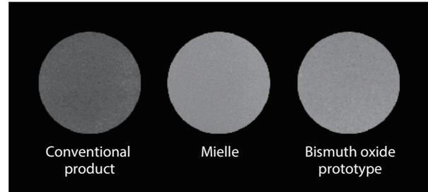
Figure 3-24 X-ray photographs of 1-mm-thick pellets of MTA cement
