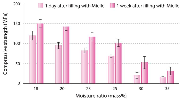
Figure 3-12 Compressive Strength of Mielle by Moisture Ratio
