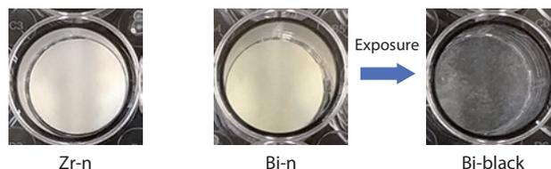
Figure 5-3 Prototype MTA cement containing bismuth oxide (before and after light exposure) and Zr-n
