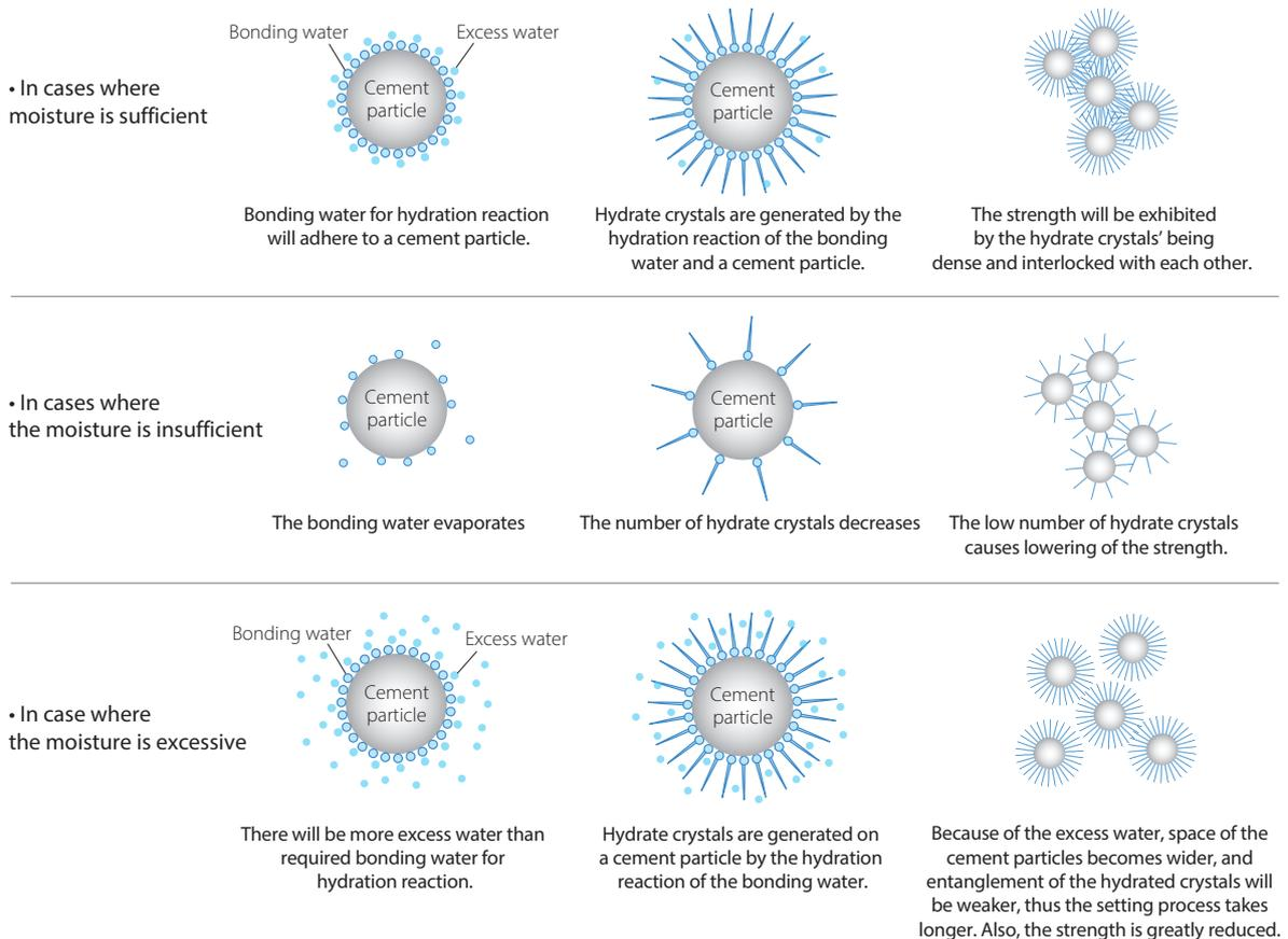
**Figure 2-3** The Difference in Hydration Reaction Caused by the Amount of Water
