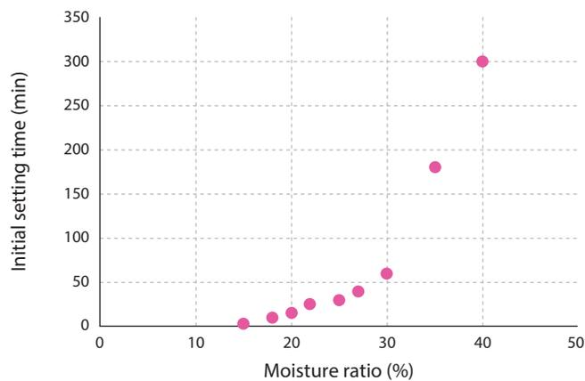
Figure 3-4 Relationship between moisture ratio and initial setting time
