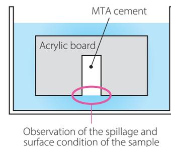
Figure 3-5 Diagram of disintegration test
