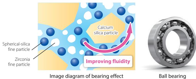
Figure 3-1 Image of Bearing Effect
