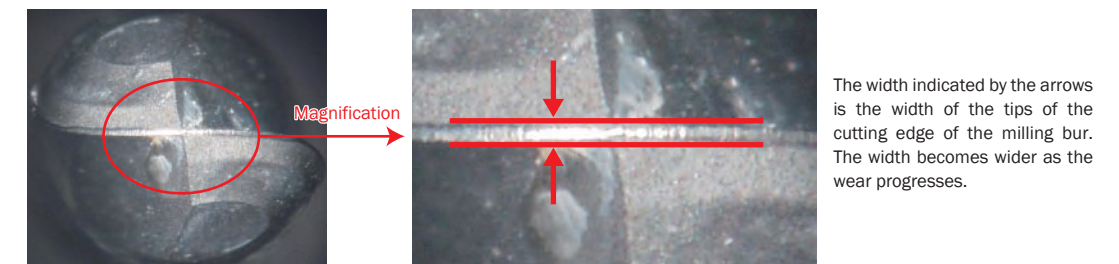
Figure 34. Evaluation Method of Wear of Milling Bur
