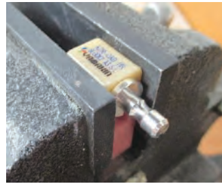
Figure 27. Block Set on the Drilling Machine
