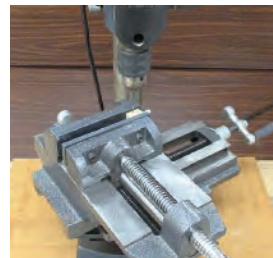
Figure 29. The Block Being Drilled
