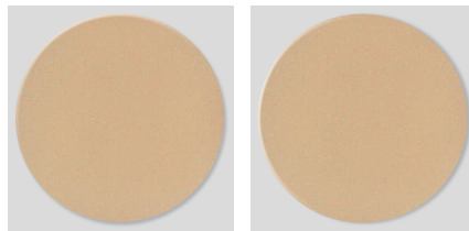
Figure 24 Colour difference of iGOS Universal before and after being immersed (Left: before being immersed Right: after being immersed)
