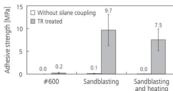
Fig. 1: Shear adhesive strength of each zirconia specimen
