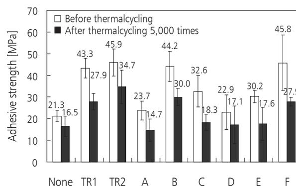
Fig.1 Effects of thermal cycling on adhesive strength
