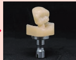
4 Completion of Milling (L size)
