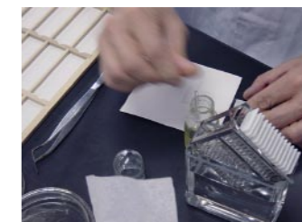
A Glass Cover is Installed to Complete a Permanent Preparation
