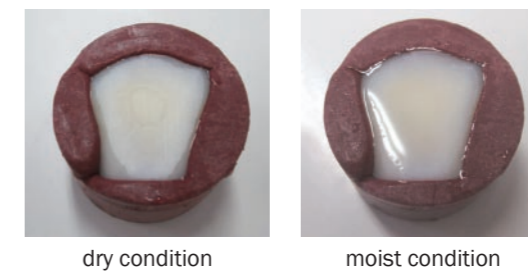
Figure 5 Test specimens for adhesion test (dry condition and moist condition)
