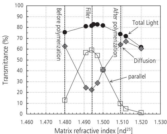
Figure1: Characteristics of Optical Transmittance of filler (firing temperature: 1100°C; content by percentage: 50 wt%)
