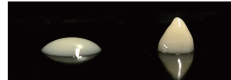
Figure 18 Formability of "Z Fill" Flowable type resin (Left: Flow Right: Low Flow)
