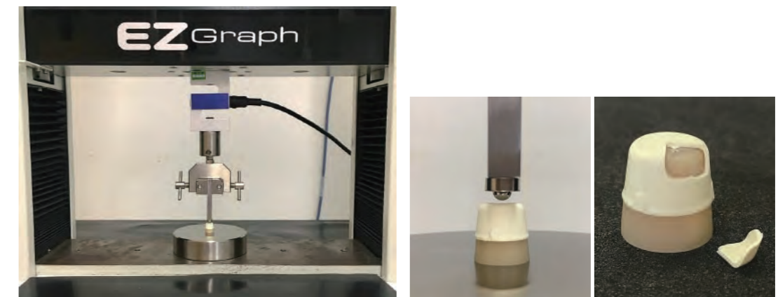
Figure 15 Test specimen for breaking-strength test assuming a single crown coping, and the tester
