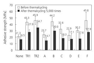
Fig.1 Effects of thermal cycling on adhesive strength
