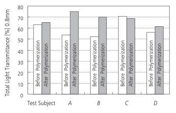
Figure: The influence of resin polymerization on changes in transmittance under total light transmittance
