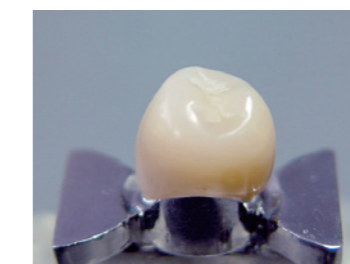
No Cracks after Thermal Testing in Hot and Cold Water over 5,000 cycles
