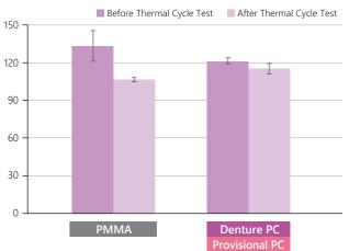
Thermal cycle test conditions: 5000 time of immersions in distilled water at 4°C and 60°C for 1 minute each
